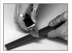
When sharpening or cutting, always push the knife blade away from you or other people. Several types of sharpeners are now offered for serrated and non-serrated blades. David Kowalski photo. to use cutting boards so blades are not chipped or bent and counter tops are not damaged. They will learn that French chef knives, steak knives, paring knives and bread knives work best when used for their special tasks.
